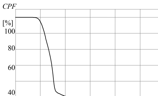
Fig. 21. Cumulative probability function CPF measured at the 110kV bus of the perturbing end-user
