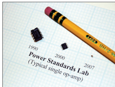
Fig. 1. Reduction in component size. Smaller components reduce costs in several ways: smaller printed wiring boards, smaller plastic packages, even smaller power supply requirements. The packages shown are, from left, through-hole DIP, surface mount, and BGA or ball-grid-array.
