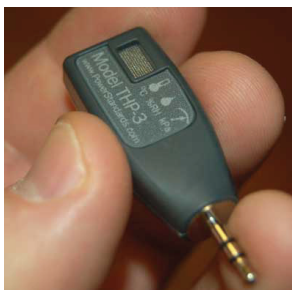
Fig. 5. Probes for parameters that may be related to power quality are included: Temperature, Humidity, Barometric Pressure, etc. A GPS satellite receiver can ensure precise timing.
