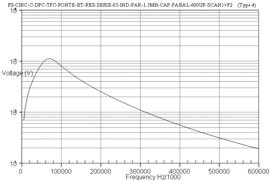
Fig. 24. Output voltage of test setup, applied to CVT, with series 0.5\Omega resistance, shunt 1.5\text{mH} and 600\mu\text{F} capacitance for passive reactive compensation.
