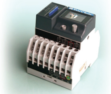
Fig. 4. Prototype of the three-phase, voltage-and-current, 61000-4-30 Class A power quality monitor. The digital camera influence can be seen in the SD memory card, which holds up to 2 000 MB of data. Standard DIN-rail mounting means installation is cheap and quick.
